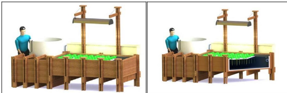
Figure 2: A 3-D drawing of the small aquaponics system (left). A cut-away view of the water tank for plants (right).
