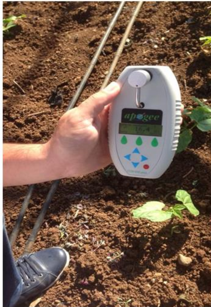
Fig. 2: Field measurements of chlorophyll content by chlorophyll meter instrument
