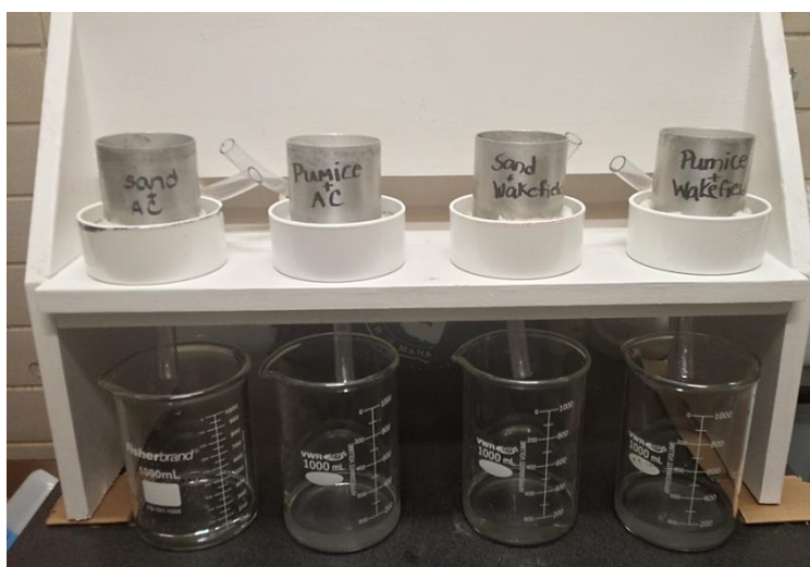
Figure 2: Column experiment setup.
