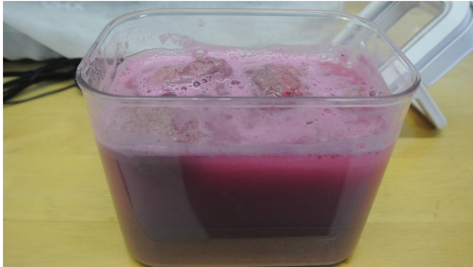
Figure 9: Then the pumice earth was added until saturation. At first it seemed to mix but then pumice sand precipitated.
