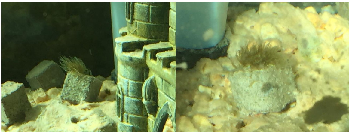
Figure 7: Close-up of the previous photograph, where algae growth can be seen on the top of a QBLOCK™.
