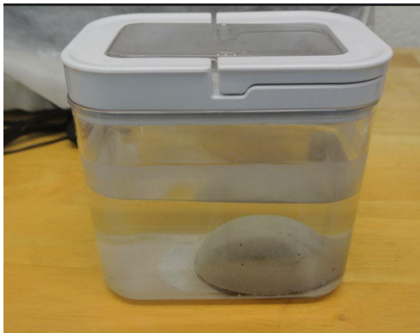
Figure 8: Purified water and a block of our material in the shape of a gray hemisphere (bottom) were placed in a transparent plastic container with a hermetic seal.
