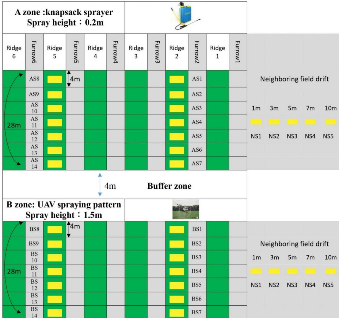
Layout of detection points for Leaf Front droplet deposition distribution
