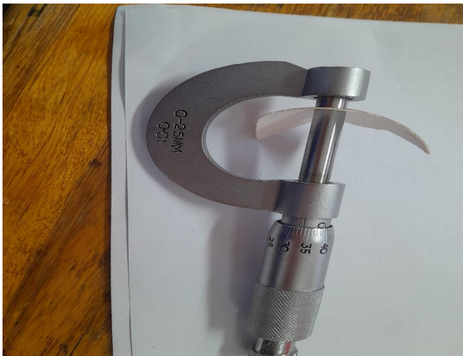
Figure 2: Egg shell thickness measurement with Micrometer screw gauge
