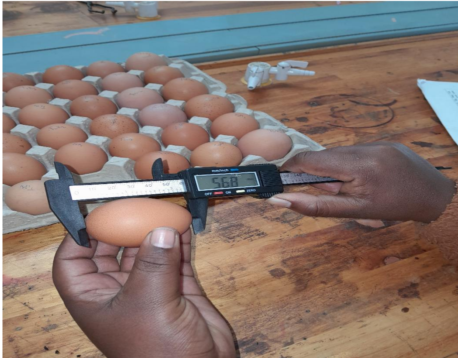
Figure 1: Measurement of egg length with Venier caliper
