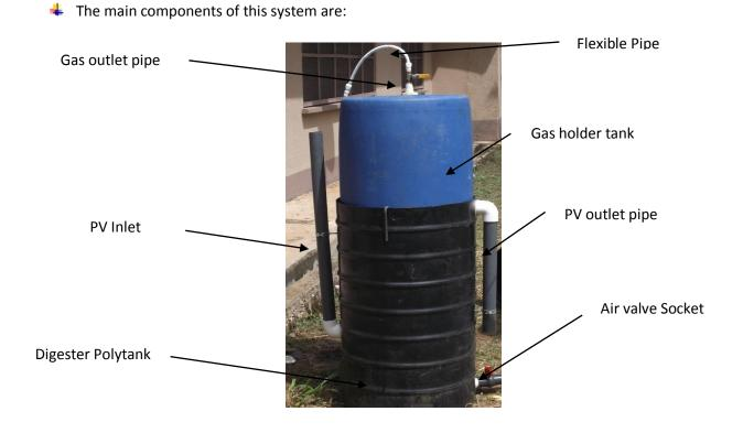
Figure 6: Complete unit digester tank
